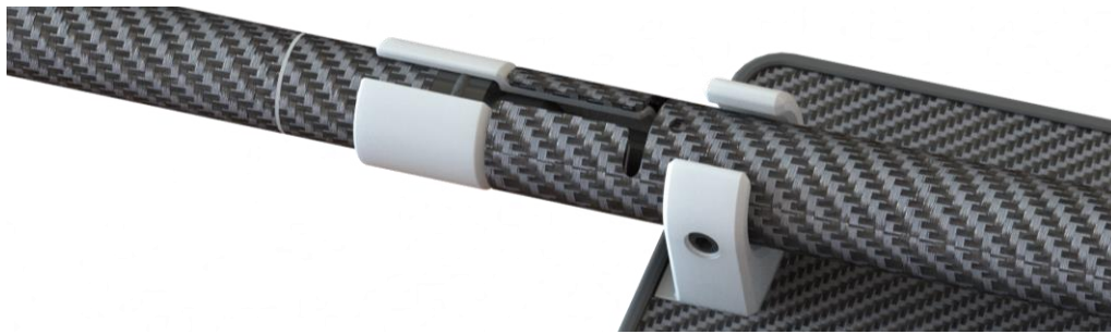
Figure 22. Mounting the RTI CT Ion chamber.
